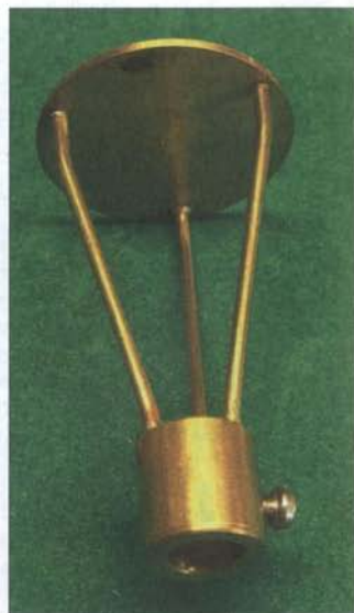
Fig. 5 - Sub-reflector with drilled sliding part
