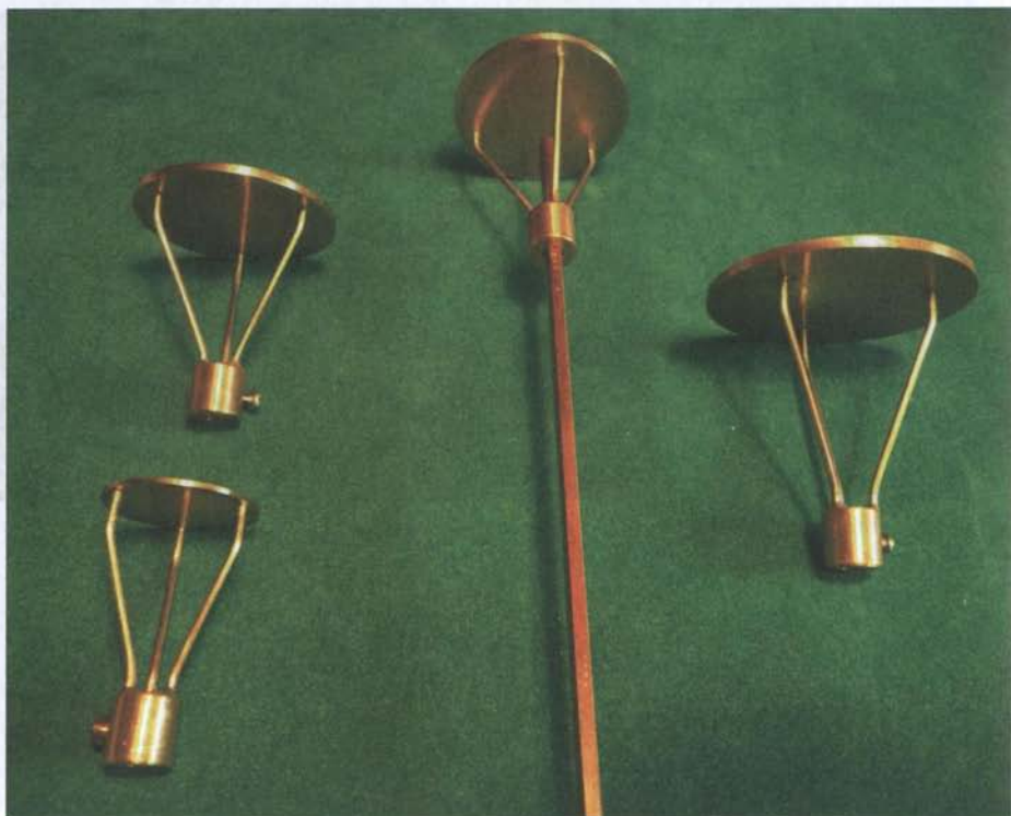
Fig. 4 – WG and different sub-reflectors with diameters from 25 to 50 mm
