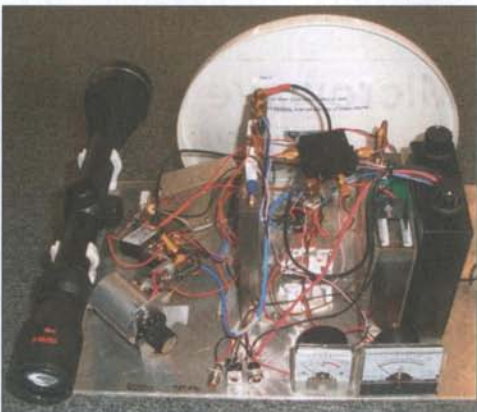
Transverter using Broadern ed-0296-2 module (single resistor mod to work as x3/amp up to 1W at 33GHz)
