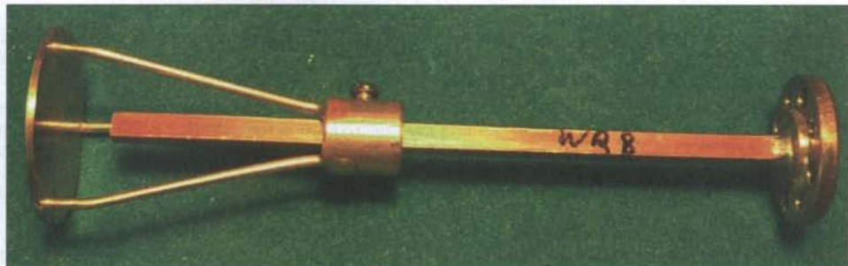
Fig. 2 - Slideable sub-reflector with WG for 490 mm dish
