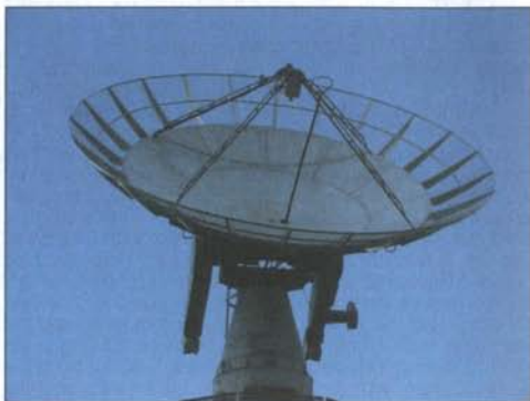
OK1KIR solid 4,5m dish mesh-extended to 6m
