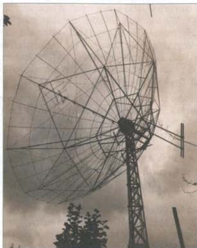
Fig. 1: 10m dish used for 2m EME in 1975 by Mr. Kumamoto, JA6DR
